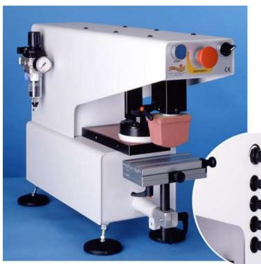
Silicon pads are widely available in various shapes and shore hardness to suit the size of the artwork to be reproduced and equally importantly the design and contours of the component to be printed.
